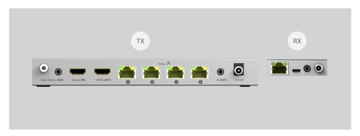
The XTND 4K (40) TPC Splitter (1x4+1) has been designed for the most modern home entertainment market requirements. This XTND is HDMI 2.0 compatible, boasting 18G HDMI interfaces, that support the latest 4K HDR video content as well as 1080p and Dolby Atmos surround sound distributed over a single Cat6 cable to 4 display locations up to 40m (131ft) away.
