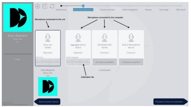
Select the microphone that you wish to use for measurements—usually the one you connected during setup. Click the bottom of the microphone's box to load the relevant calibration file. Selecting "No calibration" after clicking the context menu bypasses any compensation to the raw input stream and is not recommended. Make sure that the microphone calibration file is created for 90-degree measurements.
