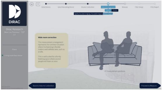
An arrangement can be chosen from the arrangement menu. In the arrangement menu, the home section has three different arrangements: Tightly focused imaging, Focused imaging, and Wide imaging, which provide 9, 13, and 17 measurement points, respectively.
