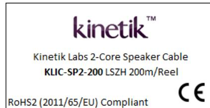
**5.Marking (ink black, every metre)** KINETIK LABS KLIC-SP2-200 OFC SPEAKER CABLE LSZH INSULATION AND SHEATH ROHS & CE APPROVED (EUROCLASS Eca) – PI/3159" + METRE MARKING
