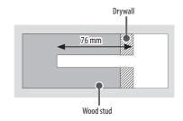
Use the Ø 4 mm drill bit for wood to drill holes with the depth of 76 mm. (Clean the drilled hole.)
