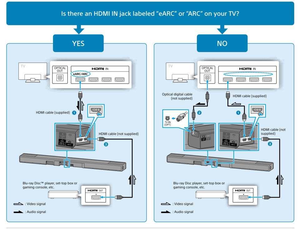
Oconnect the HDMI cable (supplied) to the HDMI OUT jack on the speaker system and the HDMI IN jack on your TV. If your TV has the S-CENTER SPEAKER IN jack, connect the S-CENTER SPEAKER IN jack on your TV to the S-CENTER OUT jack on the speaker system using the TV center speaker mode cable (supplied).
