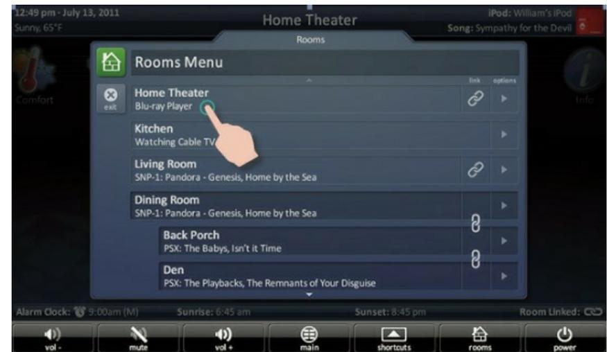
Returning the keypad to control the room where it is physically located requires accessing the **Rooms Menu** and selecting the appropriate room.
