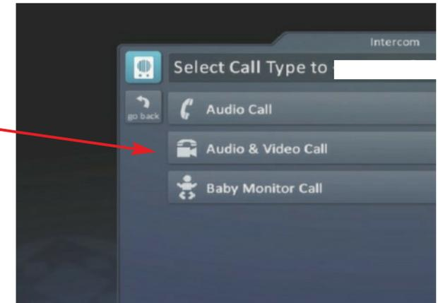
5. After selecting an option, the TDC-7100 turns the unit's camera ON (audio & video or baby monitor modes ONLY) displaying an onscreen image of the selected client (image below displays the audio/video intercom feature).
