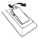
Insert two batteries correctly into the battery compartment as indicated.
