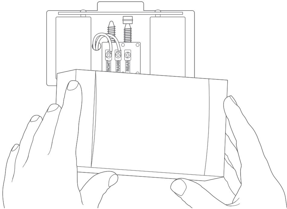
Loosen the “Front” and “Transformer” Terminals
