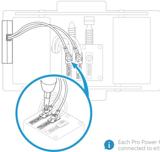
**i** Each Pro Power Kit wire can be connected to either terminal.
