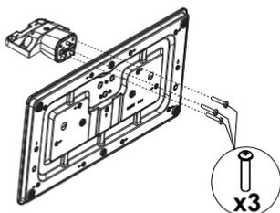
2. Place the stand(s) on the stand mounting pattern(s) on the rear side of the TV.
