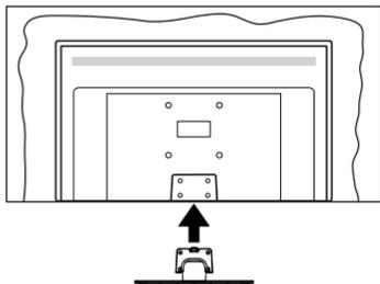
3. Insert the screws (M4 x 12 mm) provided and tighten them gently until the stand is properly fitted.
