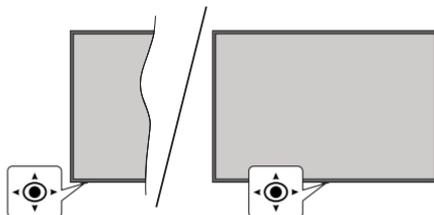
The joystick allows you to control the Volume / Programme / Source and Turn Off - On functions of the TV.
