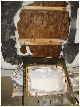
Back Box Removed—No char on floor assembly
