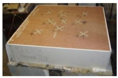
Unexposed surface after 1 hour test
