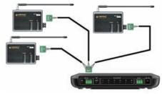
9. Should you need more than six IR Outputs, connect as many as three different MRF-350is to one RFX-250i in a daisy chain using the supplied cable.
