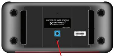
Slide off the mounting plate to reveal the RF ID# rotary switch. Check that the arrow pointer in the center of the wheel is pointed to 0, the default "interence sniffing" position. If it is not, use a small flat blade screwdriver (included) to set the RF ID# to 0.
