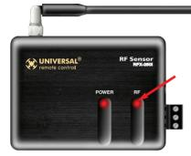
If no buttons are pressed on any remote control, no valid RF transmissions are being received. The flickering or glowing RF LED warns you that the RFX-250i is detecting RF interference generated or reflected near this location. MOVE the RFX-250i to a new location.
