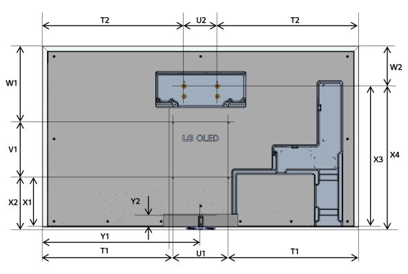
Note: flush-fit wall mount bracket (included with TV) attaches to points on the TV relating to T2, U2, W2, X3, X4 measurements. These points do not translate to attach points on the wall – the bracket has multiple options for securing to wall as shown in diagram. Use the included wall mount guide paper to position the bracket on the wall.
