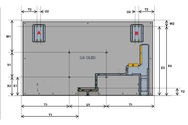
Note: flush-fit wall mount brackets (shown left, included with the TV) attach to points on the TV relating to measurements indicated in the table above and as indicated by A and B in the TV diagram. These points do not translate to attach points on the wall – the brackets have multiple options for securing to wall as shown in diagram. Use the included wall mount guide paper to position the brackets on the wall and then select drill points.
