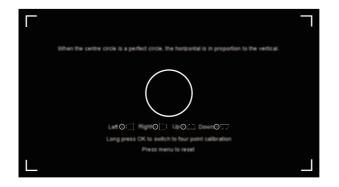
Four-point calibration: press button to move focus and choose a point you need to adjust. Press
