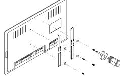
Find the correct bolts from the accessory pack that fit the holes on the back of the screen. Use these to attach the vertical bars, orientated as shown, utilising the provided washers, bolts and spacers (as required). If necessary, plug in the HDMI adaptor into the back of the screen.
