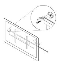
Thread the securing rod through the wall plate as shown. To lock it in place insert the M4/12 bolt through the rod and screw the nut on tightly. A small padlock can be used instead for extra security (not supplied).
