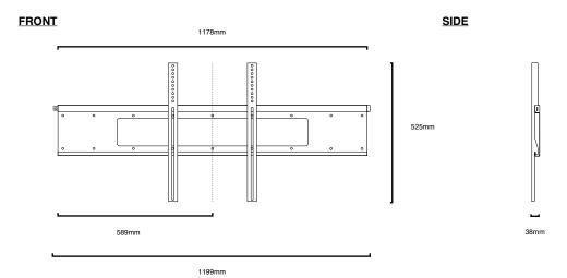
Horizontal fixing range: 100 - 1100mm Vertical fixing range: 150 - 470mm Maximum screen weight: 80kg
