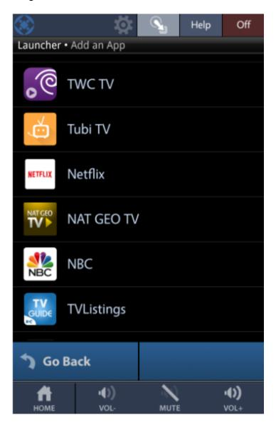
Once an app is added to the MX-HomePro App Launcher, the app can be removed by pressing and holding the app for five seconds.
