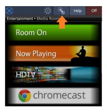
Selecting the App Launcher button results in the display of a ribbon allowing the embedding of third-party manufacture's mobile applications within the MX-HomePro Mobile application.
