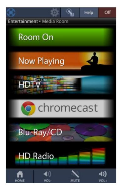
Use this screen to select the source and control the volume in your room. Use the OFF button to turn the devices in your room off. Pressing HELP at anytime provides assistance when controlling the room.
