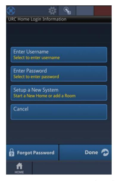
When launching the MX-HomePro Mobile Application for the first time, your mobile device needs to be connected to the same local Ethernet network that your MX-HomePro H500 Hub is connected to. You cannot be connected to a mobile broadband network for the first time discovery and connection to your system.
